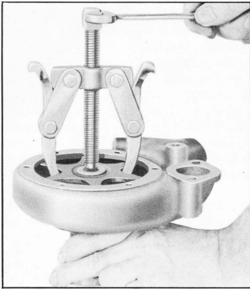
Figure 2-42—Removing Pump Impeller
