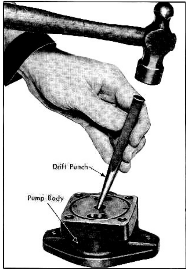
Fig. 7-20 Removing Shaft Bearing
