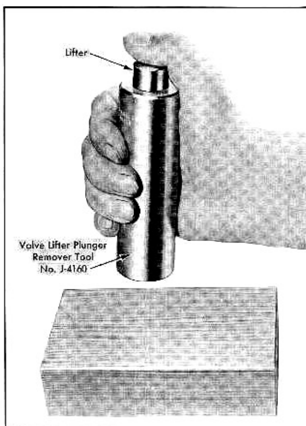
Fig. 10-14 Removing Stuck Plungers From Body
